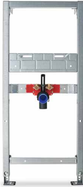
Washbasin frame Standard # WD2001 000 000 Compatible with Duravit washbasins, with the standard attachment dimensions: Angle valve distance 80–150 mm, threaded bolt distance 280 mm or 150–240 mm in the inset slot. Attachment dimensions can be configured via a metal crossbar. Infinitely adjustable crossbars.
