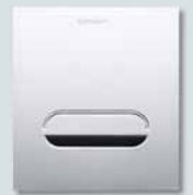
DuraSystem® actuator plate A2 # WD5006 023 000 battery-operated # WD5007 023 000 mains operation with infrared proximity electronics die-cast zinc high-gloss chrome
