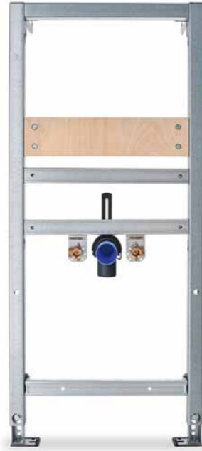
Washbasin frame Special # WD2002 000 000 Compatible with Duravit washbasins, with different attachment dimensions: Angle valve distance 80–290 mm, hanger bolt distance 50–330 mm, e.g. for handrinse basins with hanger bolt distance < 150 mm or washbasins with a pedestal. Attachment dimensions can be configured via a wooden crossbar. Infinitely adjustable crossbars.
