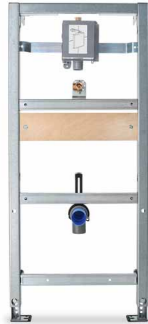
Urinal frame for concealed flushing valve # WD3002 000 000 Cross bar with concealed plastic housing and quick-fitting system. Infinitely adjustable crossbars. Suitable for dry-wall installation.
