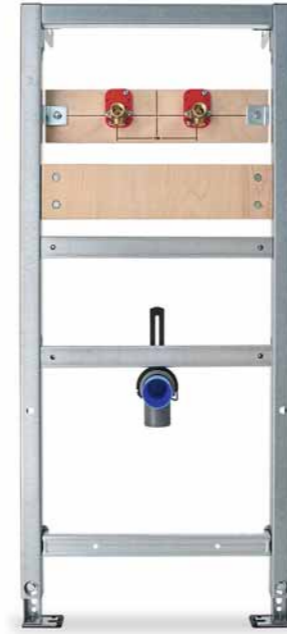
Washbasin frame for wall-mounted faucets # WD2003 000 000 For ceramic washbasins without tap hole, wall-mounted faucets can be attached via a wooden crossbar. Infinitely adjustable crossbars.
