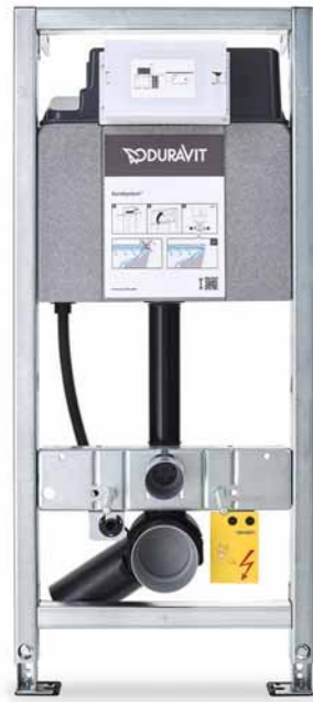
Toilet frame Standard # WD1001 000 000 In-wall cistern, maximum flushing volume 9.0 l, insulated against condensation, incl. SensoWash®-prepared. Operated from the front. Suitable for dry-wall installation.
