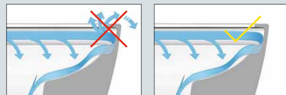
Splash-free flushing thanks to a perfect flush flow
