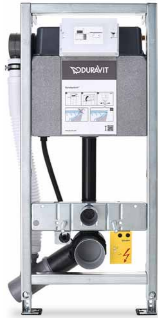
Toilet frame with manual odour extraction # WD1002 000 000 In-wall cistern, maximum flushing volume 9.0 l, insulated against condensation, incl. SensoWash® preparation. Operated from the front. Suitable for dry-wall installation.
